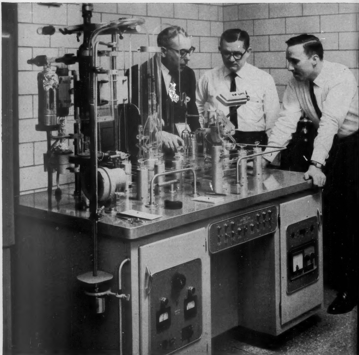
Exact measurement of hydrogen, oxygen and nitrogen in metals is made in a few minutes with the Serfass Gas Analyzer. It determines traces of these gases down to 0.1 part per million . . . can be used both for vacuum fusion and hot extraction. Here, a Fisher Technical Specialist (left) discusses a problem with the Assistant Chemist and Chief Chemist of Vanadium-Alloys Steel Co.
